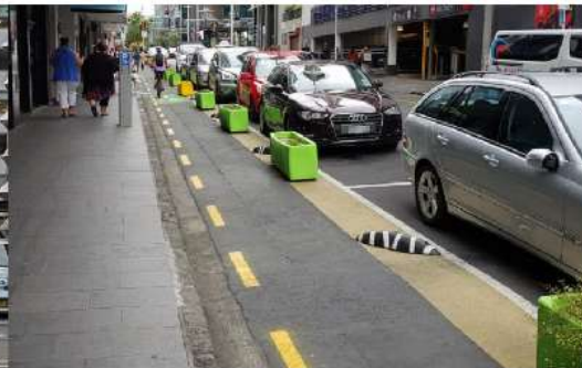
Figure 23 Planter boxes used to separate cycleway, source: NZ Ministry of Transport
