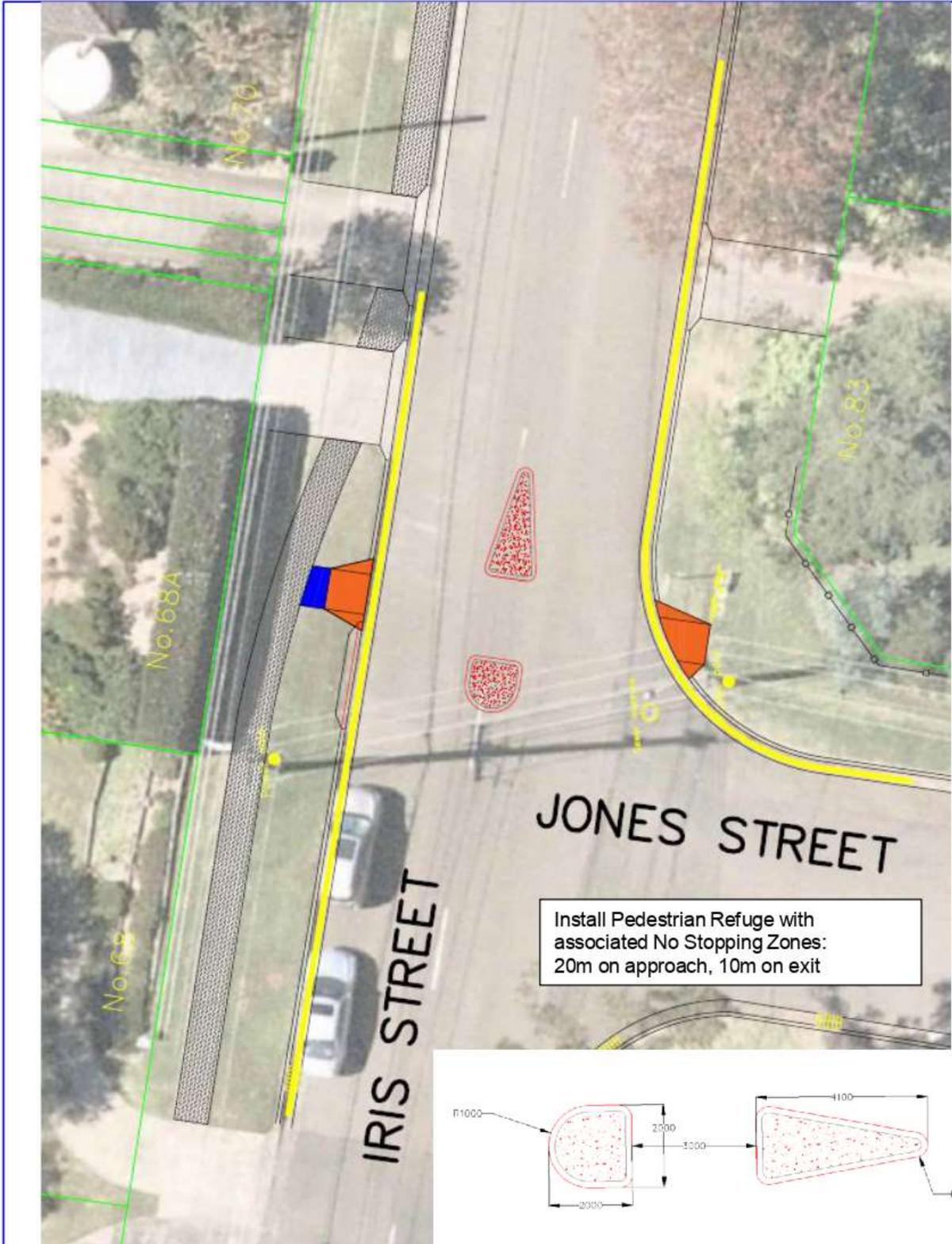
Install Pedestrian Refuge with associated No Stopping Zones: 20m on approach, 10m on exit
