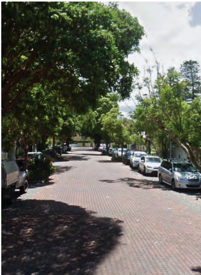
SMITH STREET, MANLY// ASPECT STUDIOS Permeable paving and trees within carriageway.
