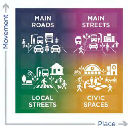
Image 1: Movement and Place Framework demonstrating the prioritisation of movement and place functions in different locations. Source: Transport for NSW Movement and Place - https://www.movementandplace.nsw.gov.au/place-and-network/identifying-street-environments
