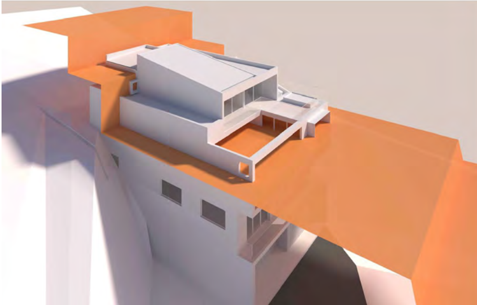
Figure 1 – excerpt from drawing HS01 showing the 8.5m building height plane, the proposed building and the location / extent of elements exceeding the building height plane
