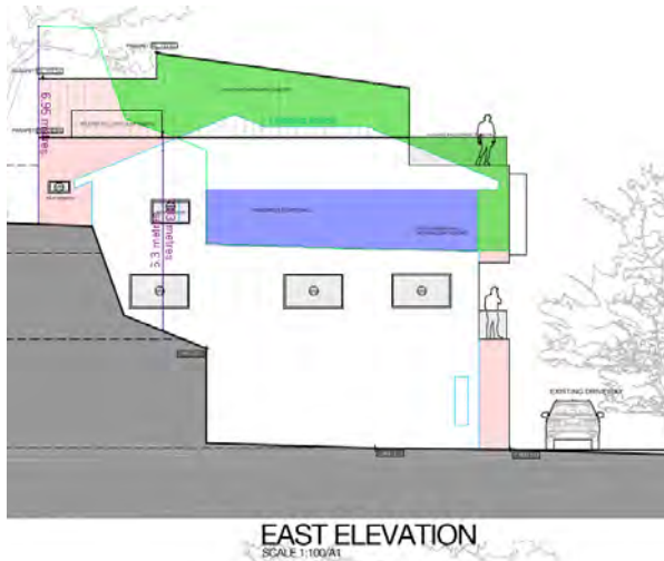
Figure 4. Eastern side boundary envelope breach (extent indicated by green shading, existing approximate breach indicated by blue shading).
