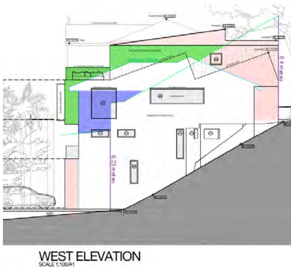
Figure 5. Western side boundary envelope breach (indicated by green shading, existing approximate breach indicated by blue shading).
